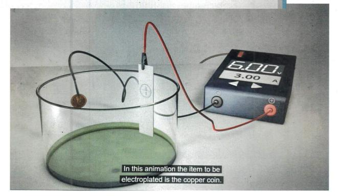
There are several factors that could affect the mass of the electroplated metal on the coin, for example: current, voltage, concentration of solution, temperature, surface area of metal coin in solution and duration of electroplating.
